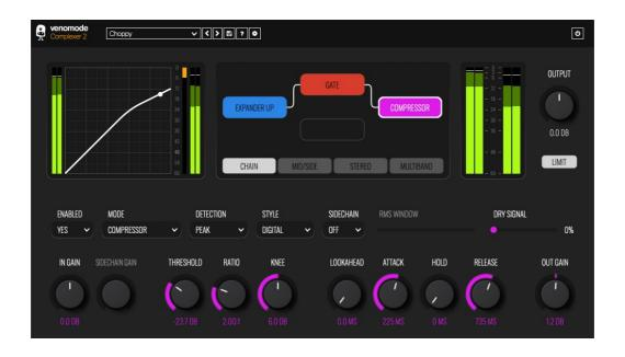
Complexer 2 is a multi-stage dynamics processor, featuring three independently controlled dynamics processors, each with a choice of six different modes. Each of the three processors can be configured as an upward or downward compressor, an upward or downward expander, a limiter, or a gate. Complexer 2 offers four different arrangements for processing: serial/parallel chaining, stereo, mid/side, and multiband. Complexer 2 is a dynamics powerhouse, letting you take complete control of your track.
